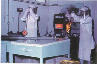
Heat-treating a gear for surface hardening
