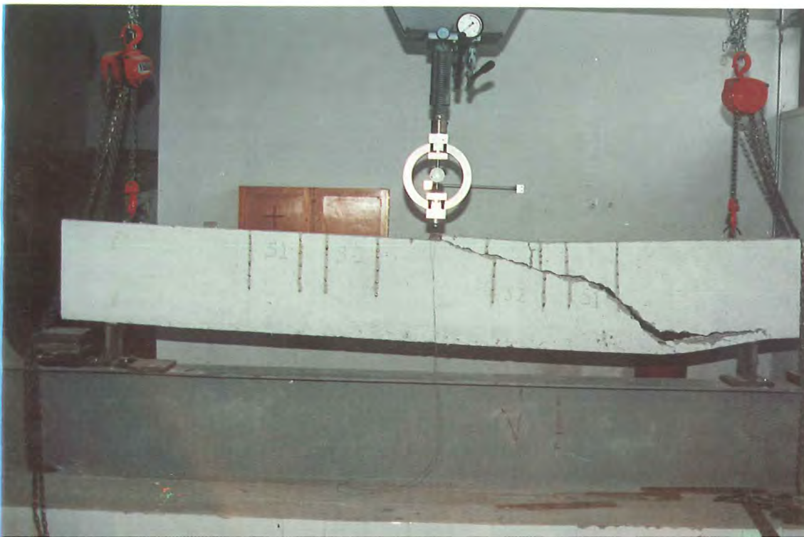
Shear Failure of a Reinforced Concrete Beam. Investigation into the shear behaviour of beams.
