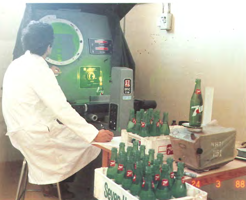
Checking the dimensional accuracy of manufacture of imported glass bottles.
