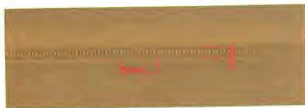
Figure 3. FBG in POF viewed with a 100x oil immersion DIC optical phase contrasting microscope. The grating period is measured as 1.06 μm a result of the formation of Talbot planes due to the imperfect suppression of the phase mask zero order.
